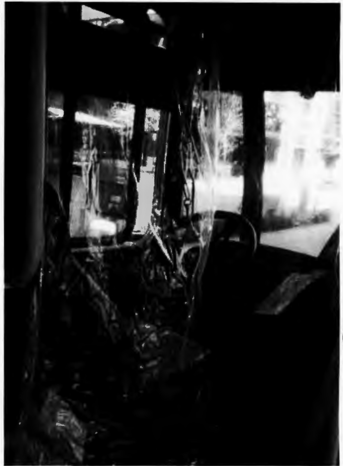
Transparent curtain separating driver's area (Source: TriMet, Oregon)
